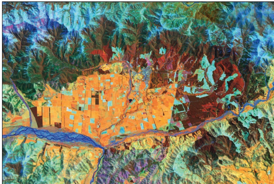
Figure 3.2 At the heart of LURNZ is a set of satellite photographs taken in three different years. This multi-spectral image shows green grass as orange, exotic forest as red, and so on, and gives much more information than a ‘natural colour’ image would. The town of Hanmer Springs is near the centre of the image.
