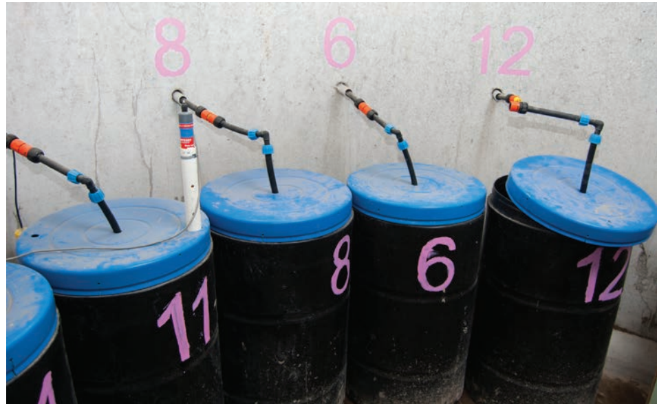
Figure 6.2 Lysimeters being used to measure nitrate flowing through soil in the Taupō catchment.
