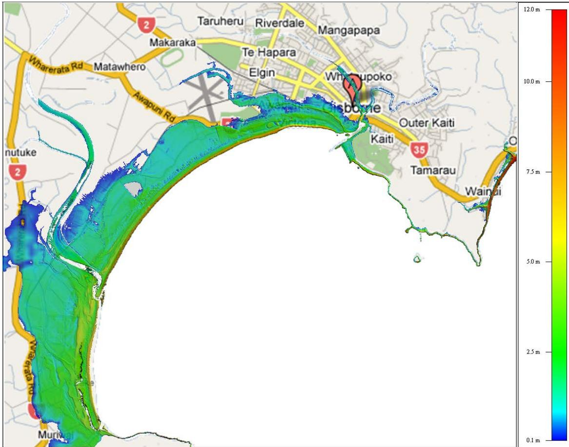
**Figure 4.10** The modelled flow depth in the Gisborne area for an MW9.0 scenario event involving rupture of the whole Hikurangi margin. The numerical simulation was performed by Wang et al. (2009) using the COMCOT model and the modelled flow depth on land is overlaid on a Google map).
