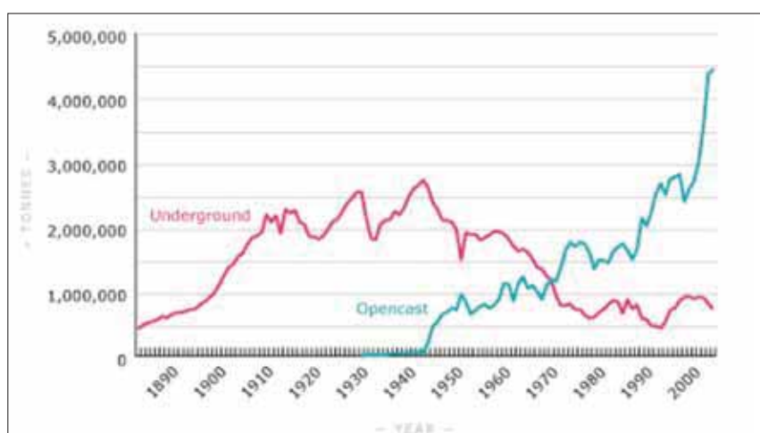
Figure 19.2: Open versus underground mining 15
