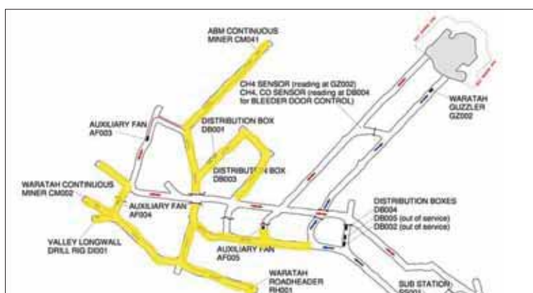
Figure 8.17: Ventilation inbye of the monitor panel 198
