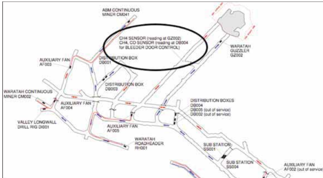
Figure 10.3: Location of hydro-panel sensors 29
