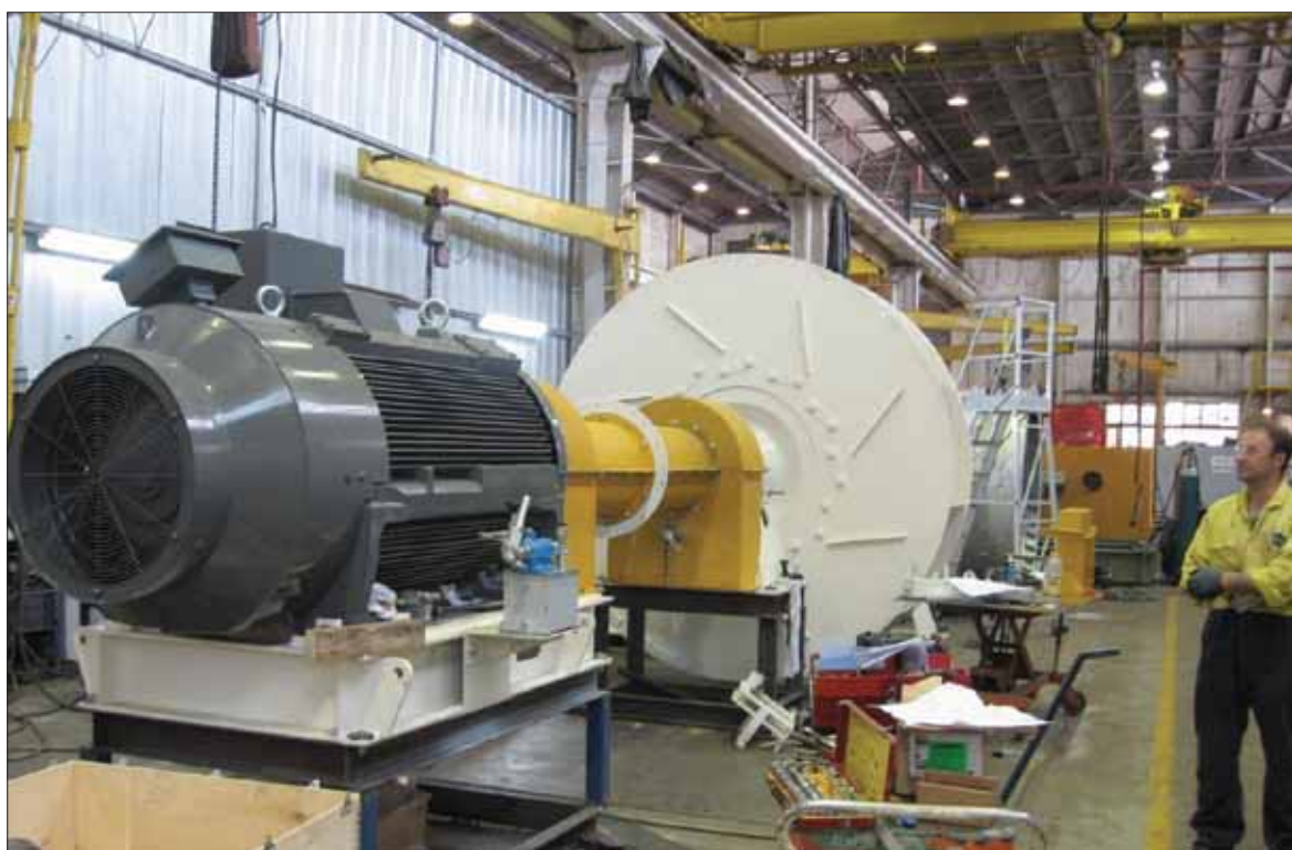
Figure 8.8: Underground fan being assembled in factory
