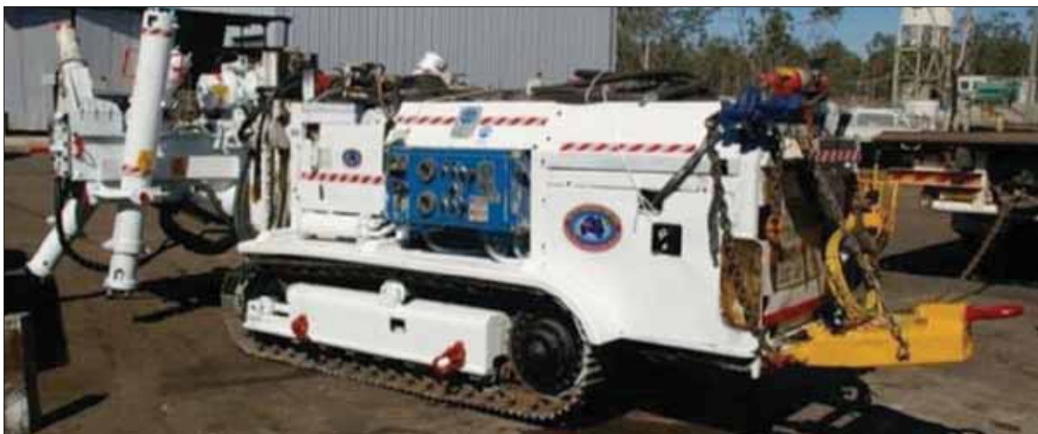
Figure 9.1: Track-mounted Boart Longyear LMC75 drill rig 31
