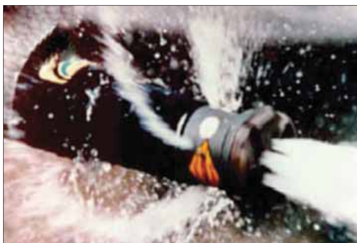
Figure 9.3: Rotating drill bit with high-pressure water 34
