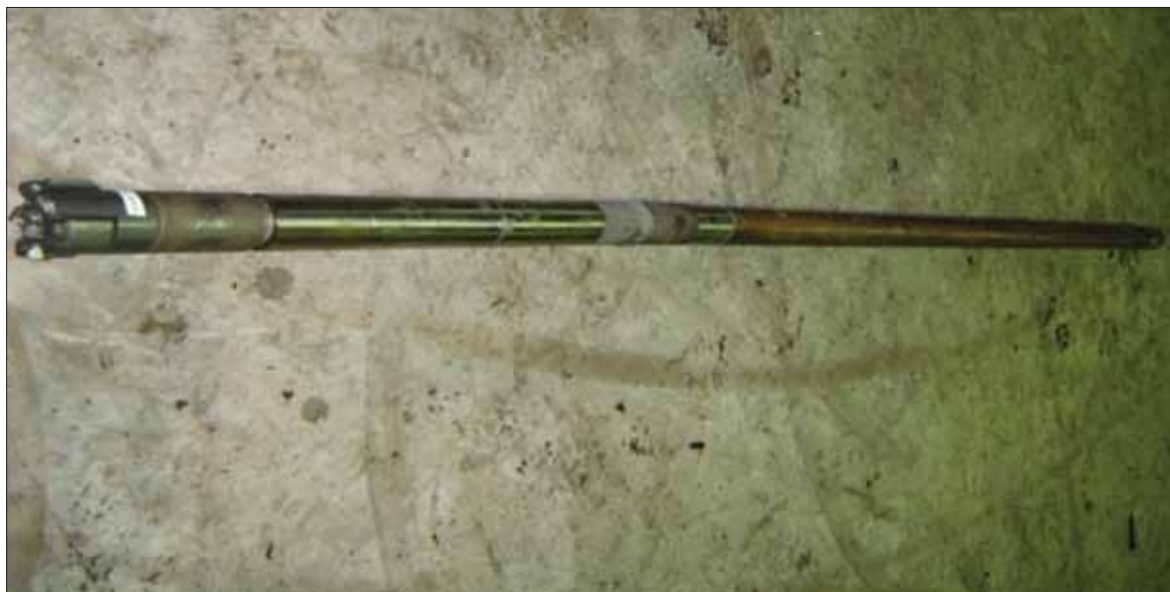
Figure 9.2: Bit, down-hole motor and assembly 33
