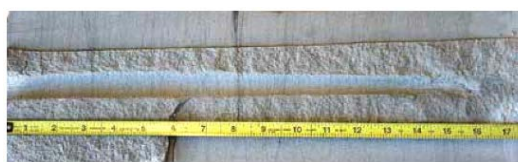
Figure 16 - Photograph of a perforation tunnel in a test slab of rock
