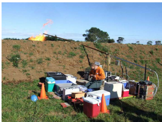
Figure 28 - Combustion zone testing set-up (from TRC report, 2012) 132
