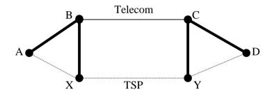
[34] In this diagram, an end-to-end circuit connects a customer's premises at point A to another of their premises at point D. The links AB and CD represent connections from the physical premises to an exchange building and the links BX and CY represent connections from an exchange to a point at which a rival TSP can pick up the transmission. This is known as a point of presence (POP).<sup>27</sup> The links
